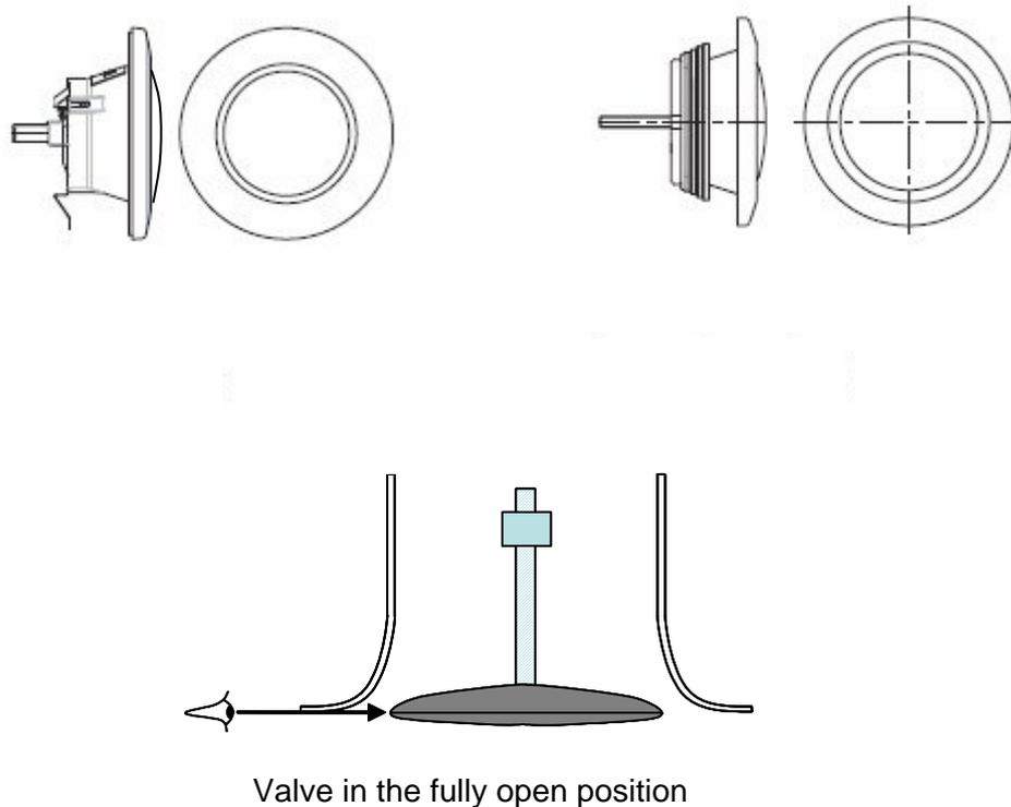
**Figure 3 - Examples of exhaust air terminal devices fully open**
