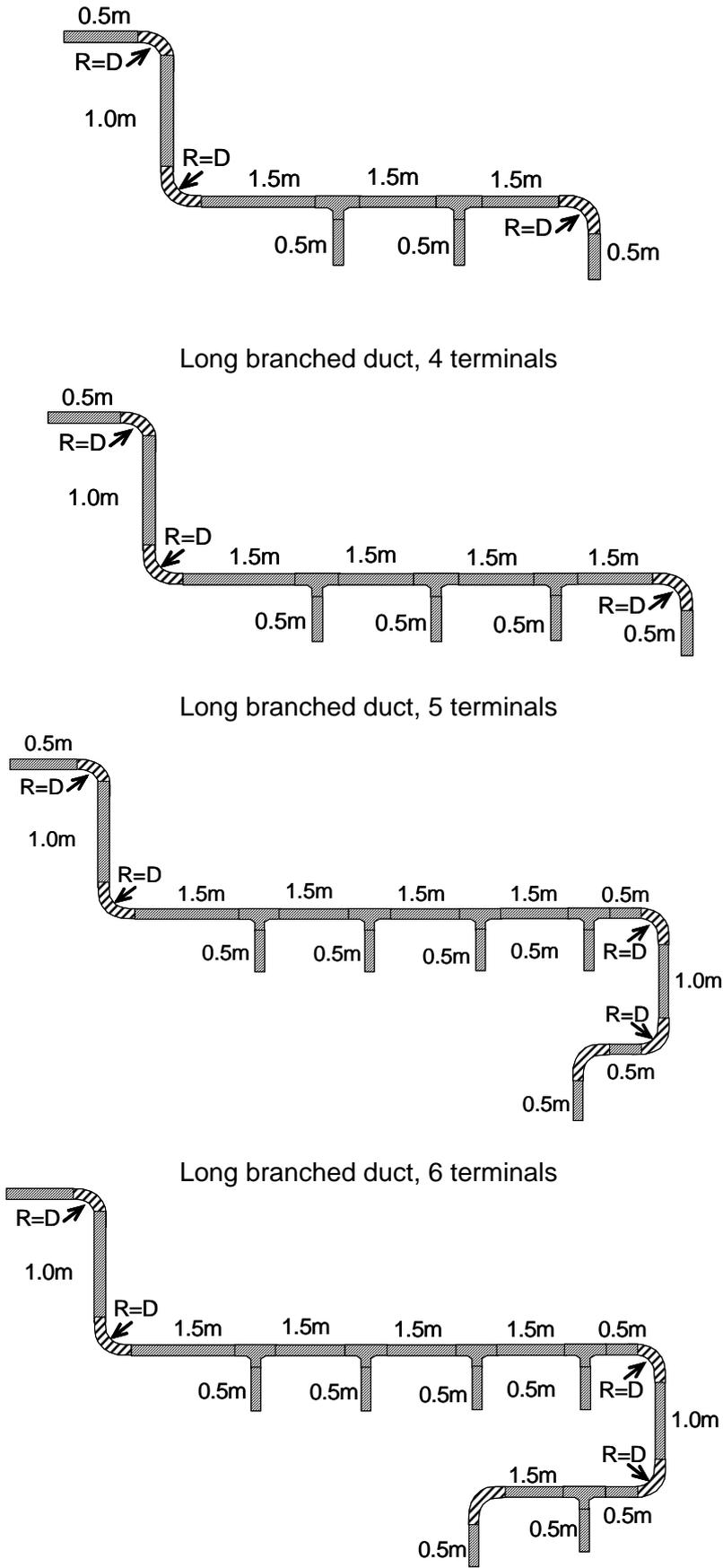
Figure 2 - Examples of duct connections
