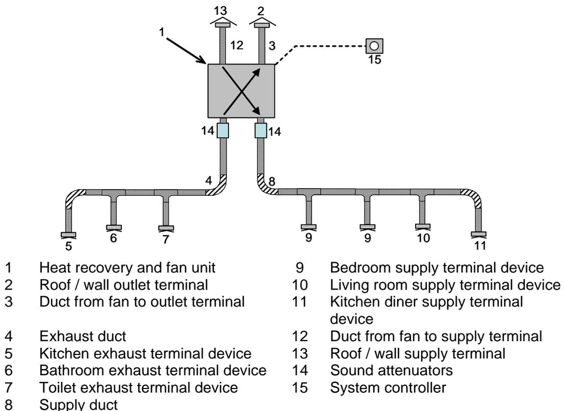
**Figure 1 - Typical components that may form part of a mechanical supply and exhaust ventilation system package with heat recovery**
