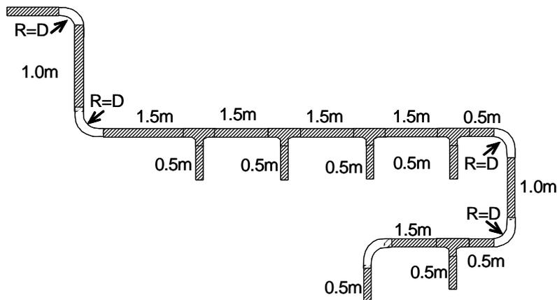
Figure 2 - Examples of duct connections
