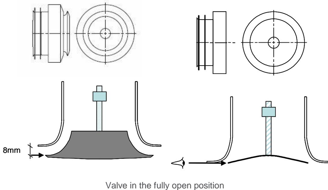
**Figure 4 - Examples of supply air valve devices fully open**
