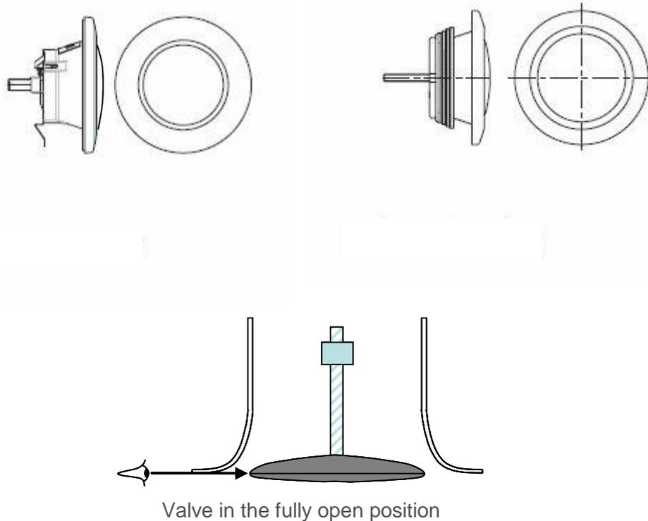
**Figure 3 - Examples of extract air valve devices fully open**
