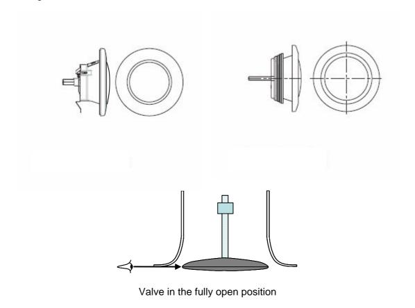
Figure 3 - Examples of exhaust air terminal devices fully open
