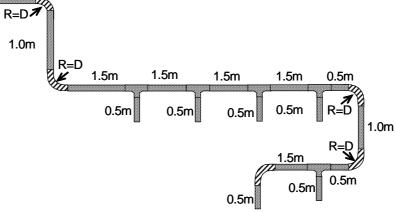
Figure 2 - Examples of duct connections
