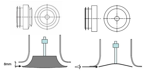
Valve in the fully open position
